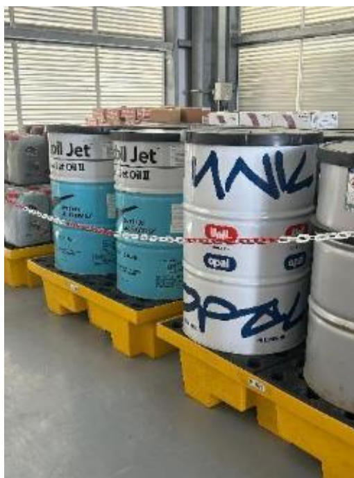
Figure 18: Secondary containment of hazardous liquids at CS1
