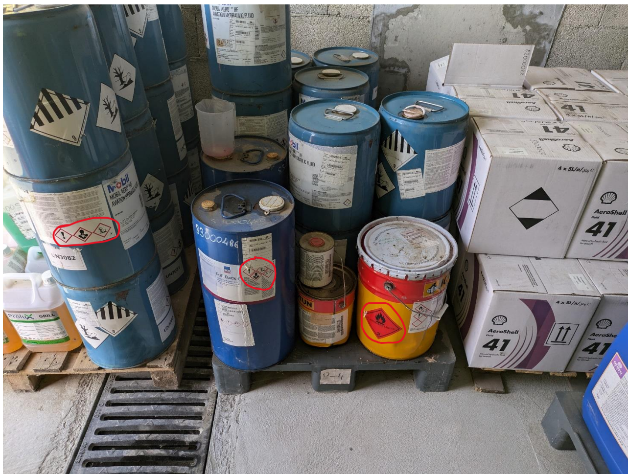
Figure 23: Example of incorrect chemical storage at MS4. Left: poison and environmental hazard. Middle: poison, corrosive and environmental hazard. Right: Flammable liquid.
