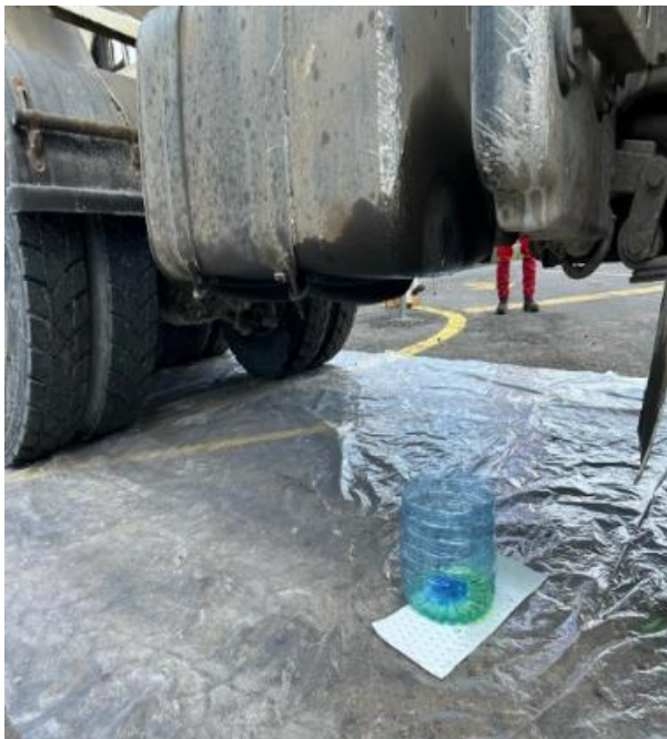
Figure 8: Diesel leaking from the concrete mixer and spill containment
