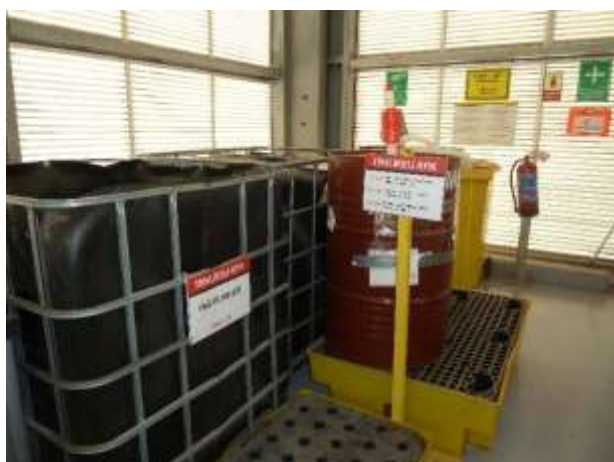
Figure 2.17: Adequate secondary containment and clear labelling of waste
