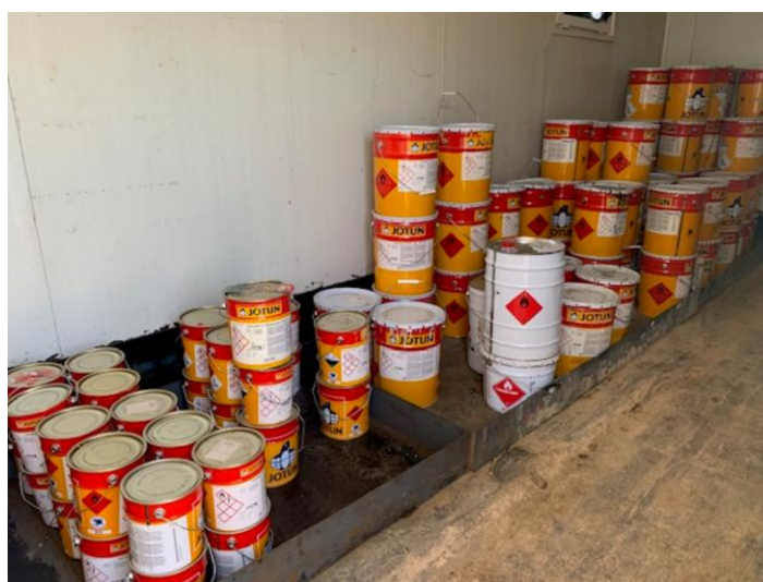
Figure 2 Incompatible chemical storage example
