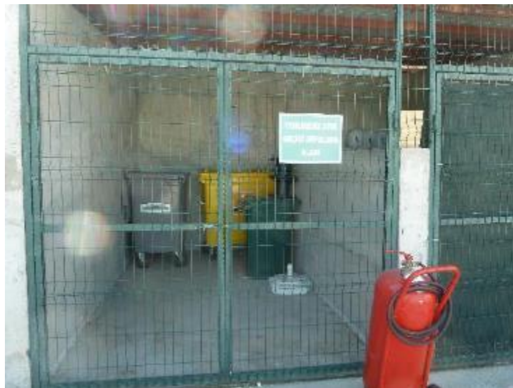
Figure 2.15 Good practice non-hazardous waste storage at CS3
