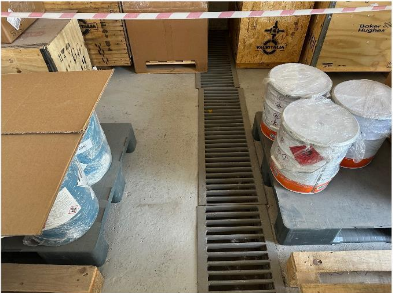
Figure 2.21 Storage of poisons and flammables together
